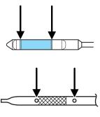
•If the oil level is **within this range**, the oil level is acceptable. **DO NOT ADD OIL**.
